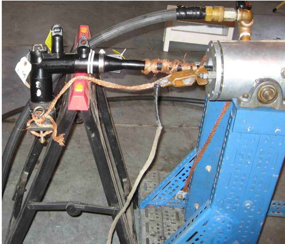
Figure 2: Test specimen inserted into water terminals.
