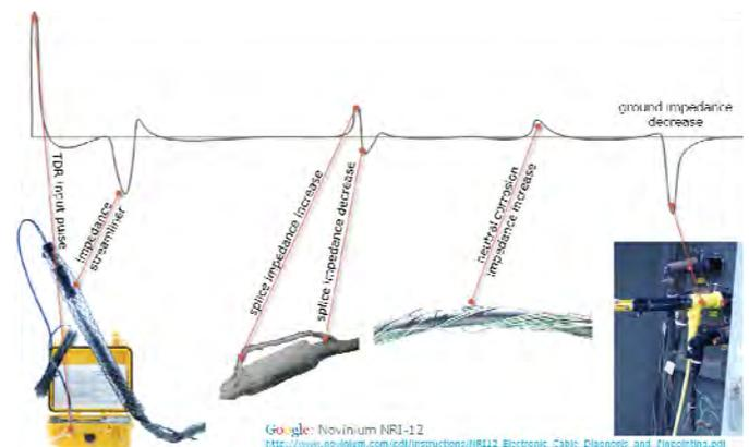
Figure 16. The principals of TDR used to identify and distinguish neutral corrosion impedance reflections from other anomalies such as splices. Virtual representations in the waveform are tied to their physical manifestations.
