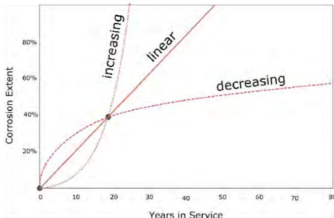
**Figure 10. Of the three possible shapes of the corrosion progression curve, the decreasing rate curve is theoretically the most likely. Survey data and anecdotal observations are also consistent with a decreasing rate curve.**
