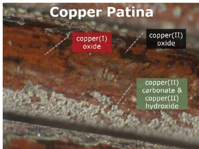
**Figure 9. Copper patina in two?? different oxidation states form a protective layer over the native copper below. The patina may be red, black, or blue-green.**
