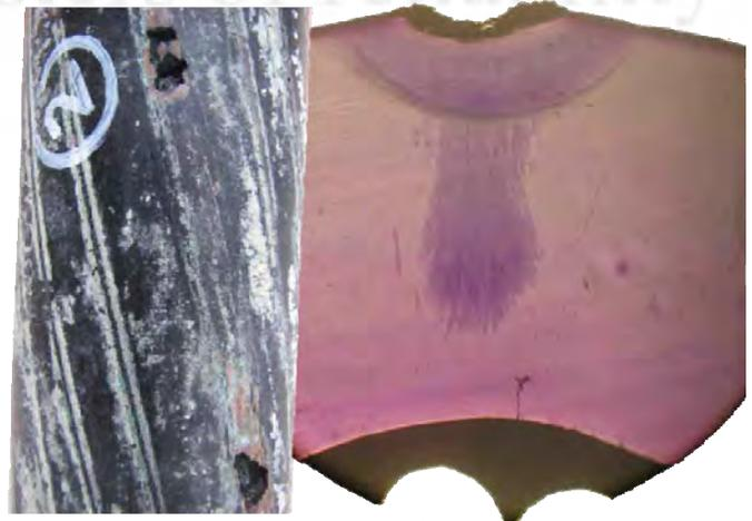
**Figure 5. Holes in the cable insulation shield were created by arcing from compromised neutrals. The erosion reached the insulation; water trees and electrical trees formed.** Images courtesy of Cable Technology Laboratories.
