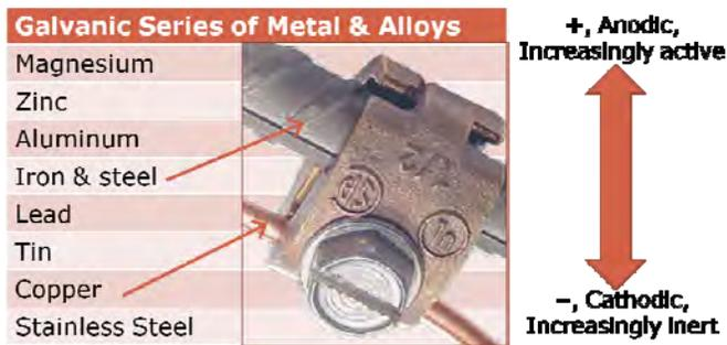
**Figure 7.** Except for stainless steel, other metals such as iron and steel are less cathodic than copper, and hence bonding copper to rebar poses no risk to the copper. Magnesium and zinc make particularly attractive sacrificial anodes.
