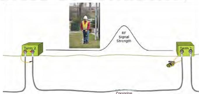
**Figure 17. Pinpointing the precise location to excavate a neutral corrosion site is best accomplished with a radio frequency locator. A transmitter is connected to the conductor and the neutral at termination 1 and a jumper cable connects the conductor and neutral at termination 2. An operator carries a receiver over the cable path. The signal increases greatly where neutrals are corroded.**
