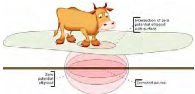
**Figure 4. The cow's hind legs are at zero potential and her front legs have a non-zero potential. If the potential difference is high enough, the cow may suffer discomfort.**
