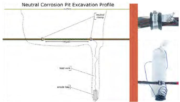
**Figure 18. Profile and hardware typically employed to correct and protect local neutral corrosion. The typical length of the repair is less than one meter. The neutral clamp is designed to make a permanent and secure electrical connection with existing neutrals which have been wire brushed and repair neutrals.**
