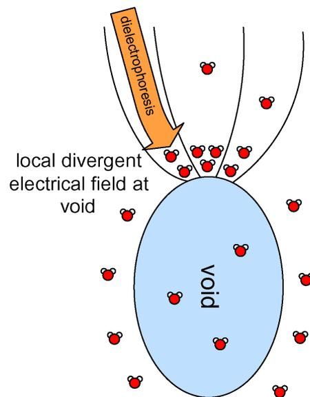
Figure 8. Model void with divergent electrical fields, dielectrophoresis, and the resulting local concentrations of water at a higher temperature.
