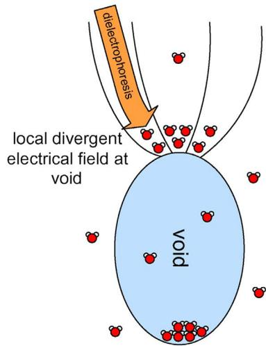
Figure 7. Model void with divergent electrical fields, dielectrophoresis, and the resulting local concentrations of water ( $H_2O$  molecules illustrated as “mouse head” icons) at a moderate temperature.
