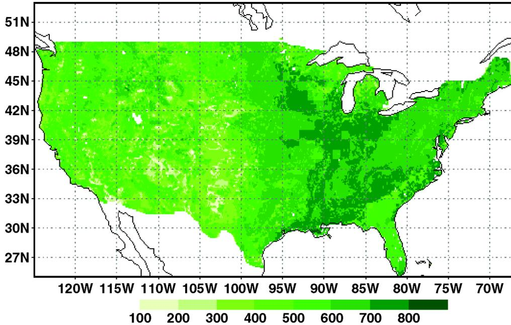
Figure 2. Water (mm) in the top 2 meters of U.S. soil in the driest month of the year (August). Depending on soil types, 700-800 mm of water represents fully saturated soil (i.e., no gaseous air present).
