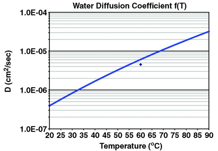
Figure 10. The diffusion of water in PE as a function of temperature. Measured values are diamonds and the model of Sletbak and Ildsatd is represented by the solid line.
