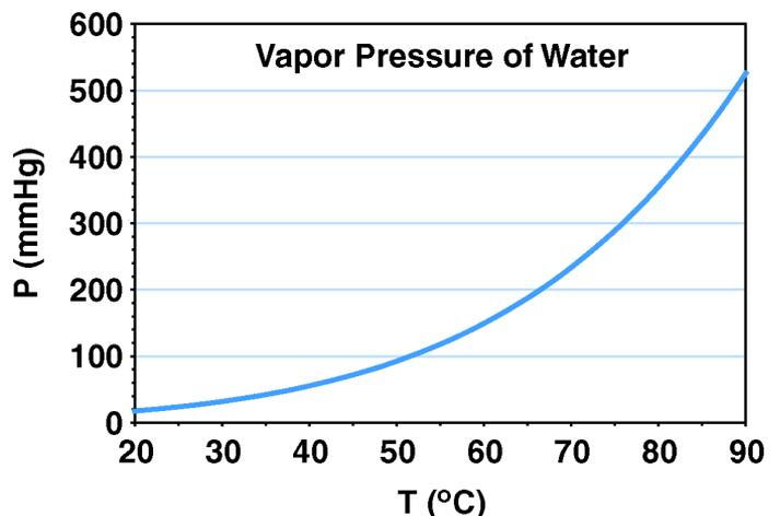
Figure 1. Vapor pressure of water as a function of temperature [1].
