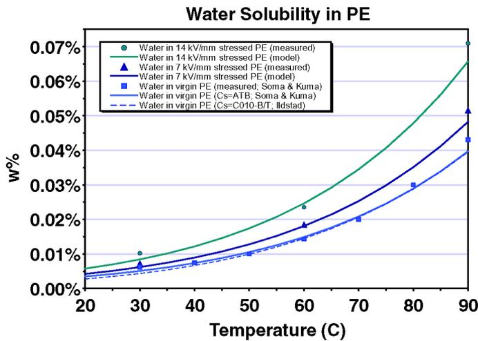
Figure 3. Water solubility as a function of temperature and divergent electrical field strength.
