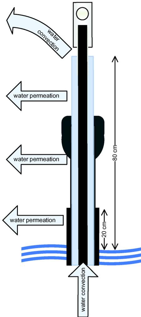
Figure 5. Termination detail of the Pélissou experiment.
