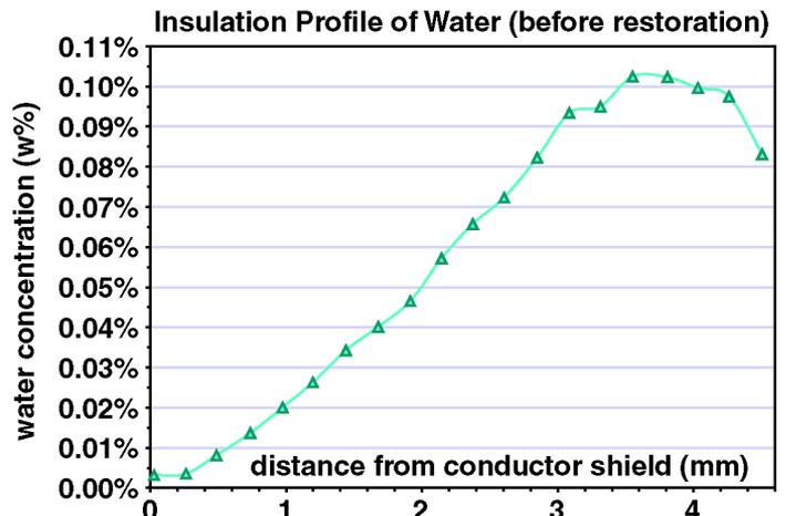
Figure 6. Water concentration profile obtained by micro-IR of 250 mm<sup>2</sup> (500 kcmil) 15kV field-aged cable.
